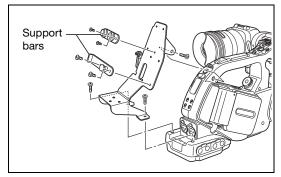
When using the optional CH-910, hook it onto the support bars and secure it with the stop lever. To detach the CH-910, press the stop lever in the direction of the arrow and pull the CH-910 off the support bars.
